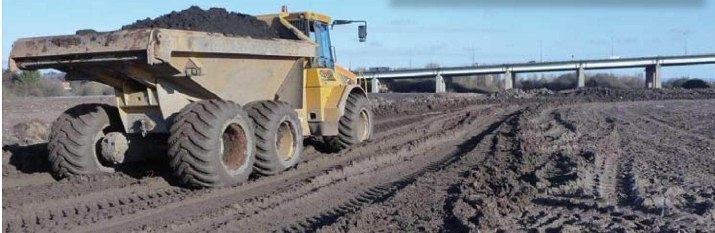
The 922s unique low ground pressure capability and impressive fuel economy make it a very environmentally friendly machine to use. Very little soil and land disturbance occur to the ground that the 922 travels over, making it a preferred choice of machine for many users in which minimal ground damage is a necessity. Such sites can include nature reserves, lake and riverside works, agricultural estates and sites of special scientific interest (SSSI's)
